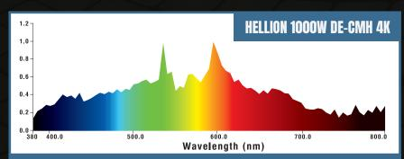
Blue-rich spectrum enhanced with continuous UV-A and far-red to drive the production of terpenes and essential oils.
