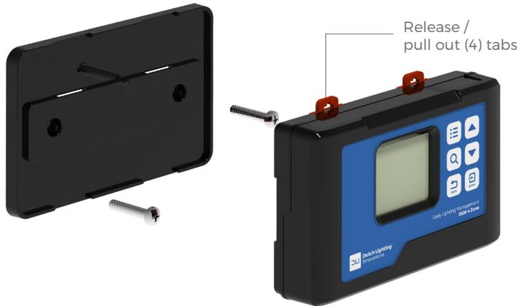
Determine where to locate the main controller. The controller comes with a simple to use DIN type bracket. Pull the 4 tabs outward to release the bracket from the unit, mount the bracket to a wall or surface, place the unit back on the bracket and press the 4 tabs back in to lock the unit in place.
