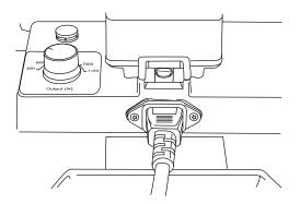
**6.** Use the control switch to adjust the light output. The output scale represents the power to the lamp.
