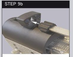
The Spreader Arm slots into the switch head in the direction shown.
