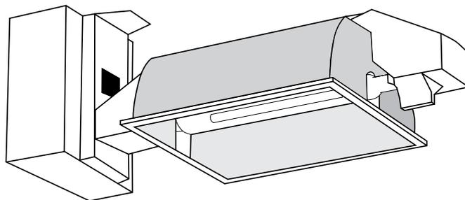
**Too hot for your crop!** *These deep-dish reflectors were designed to supplement sunlight in greenhouses during winter. Their small form causes minimal shade on the crops far beneath. However, when used in grow rooms at proximities of 60 - 90 cm these fixtures invariably overheat plants (convection and radiant heat) leading to abiotic stress, stunted growth and fewer essential oils.*
