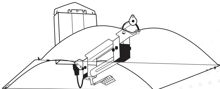
**Perfected for grow rooms.** *The Hellion's open-ended design naturally dissipates heat, prolonging lamp life. Growers can safely position the fixture as close as 45 cm from the canopy with no heat stress—all thanks to the superior reflector design and Super-Spreader. This deep, penetrating, angular and intense light drives production throughout the plant, not just the canopy leading to significantly higher yields.*
