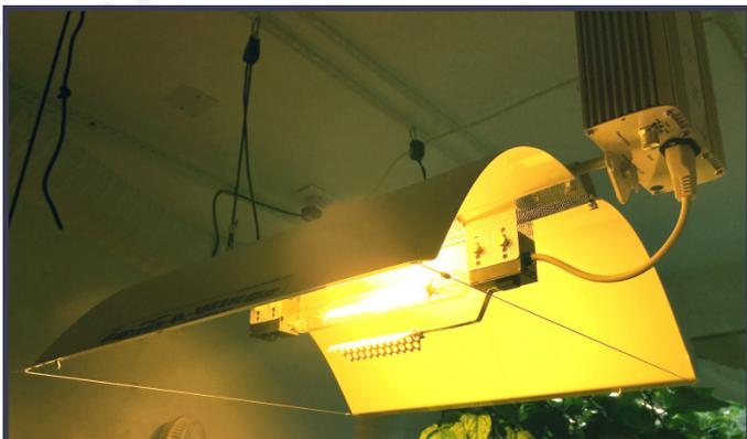
*Adjust-A-Wings reflectors enable much closer placement to the plant canopy for deeper light penetration. The patented double-parabolic reflector and Super-Spreader prevent the heat problems associated with deep dish reflectors.*
