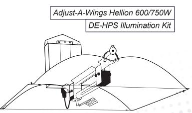
Perfected for grow rooms. The Hellion's open-ended design naturally dissipates heat, prolonging lamp life. Growers can safely position the fixture as close as 45 cm from the canopy with no heat stress—all thanks to the superior reflector design and Super-Spreader. This deep, penetrating, angular and intense light drives production throughout the plant, not just the canopy leading to significantly higher yields.
