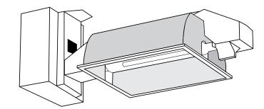
Too hot for your crop! These deep-dish reflectors were designed to supplement sunlight in greenhouses during winter. Their small form causes minimal shade on the crops far beneath. However, when used in grow rooms at proximities of 60 - 90 cm these fixtures invariably overheat plants (convection and radiant heat) leading to abiotic stress, stunted growth and fewer essential oils.
