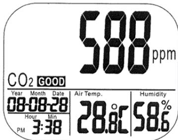
You can see the current CO<sub>2</sub>, temperature and air humidity value. Also the air quality good/normal/poor is displayed, as well as the date and time (the correct date and time still have to be set).
