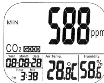
Press MIN/MAX ▼ again to read the measured maximum values (MAX).
