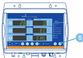
*Note: For BlueLab 2.77 EC solution, a display of 2.8 EC should be expected.*
